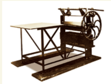
First corrugated board manufacturing machine (replica)
