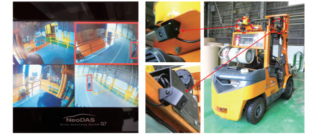
Preventing contact with vehicles through AI cameras
