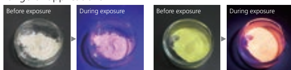
Luminescence of Gaiaphoton \gamma (when exposed to visible light with a wavelength of 410 nm)
